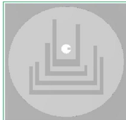
Fig.1. Geometrical representation of four U-slot micro strip patch antenna. (Dimensions are in mm).
