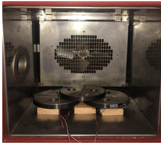
Figure 2: Carbon Fiber Composite in Climate Chamber
