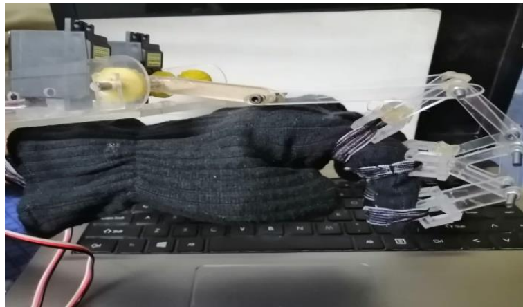
Figure 8. Exoskeleton device in flexion state
