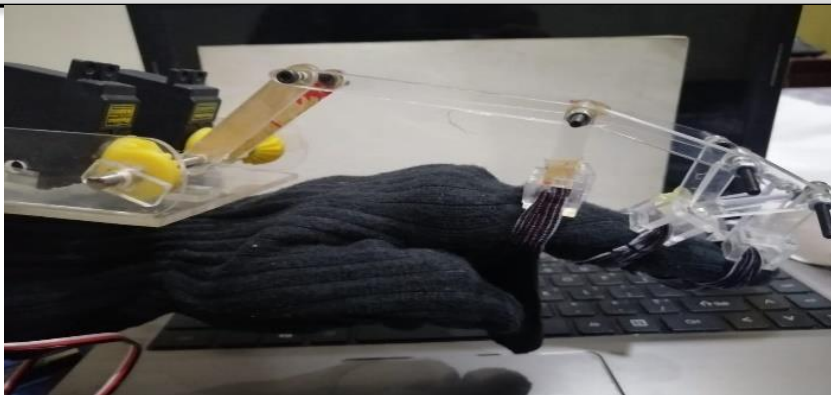
Figure 9. Exoskeleton device in extended state
