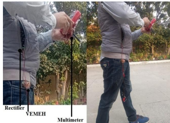
Figure11: Evaluation of the VEMEH while a person is running
