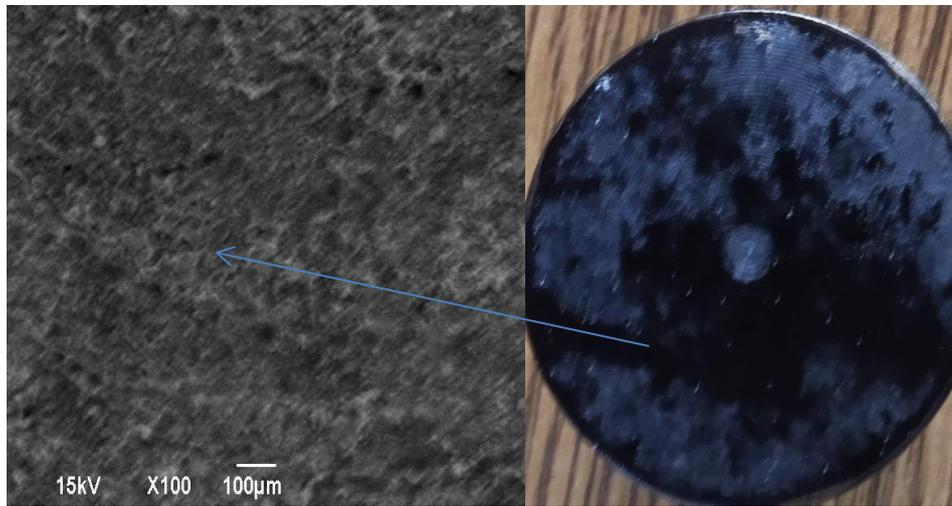
**Figure 6: SEM analysis of inlet valve at CL3000ppm**
