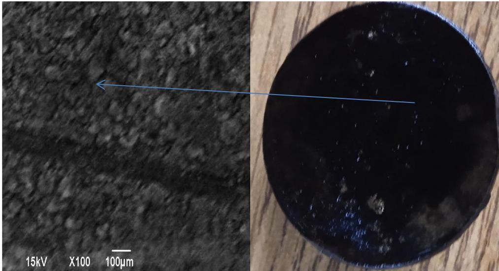
**Figure 3 : SEM analysis of inlet valve at D100**
