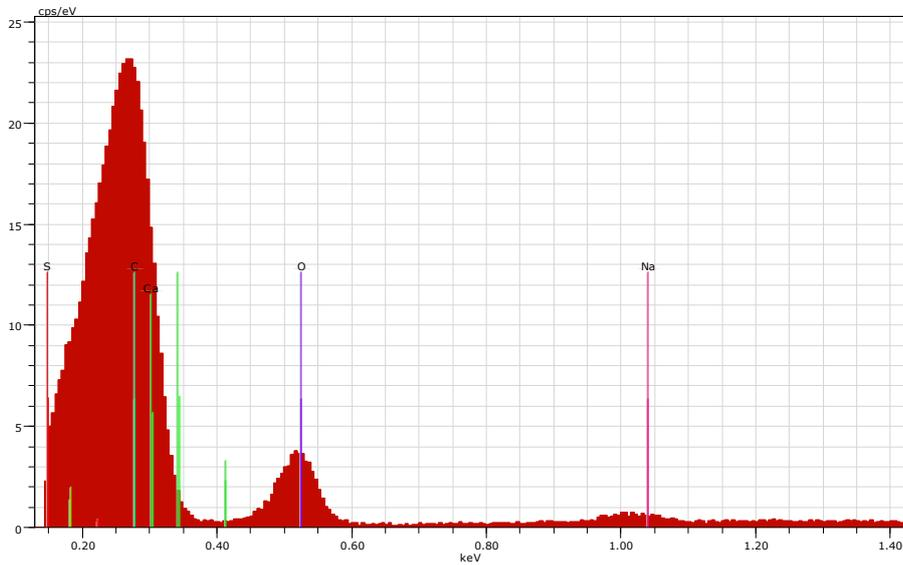
**Figure 5 : EDX analysis of inlet valve at B30**
