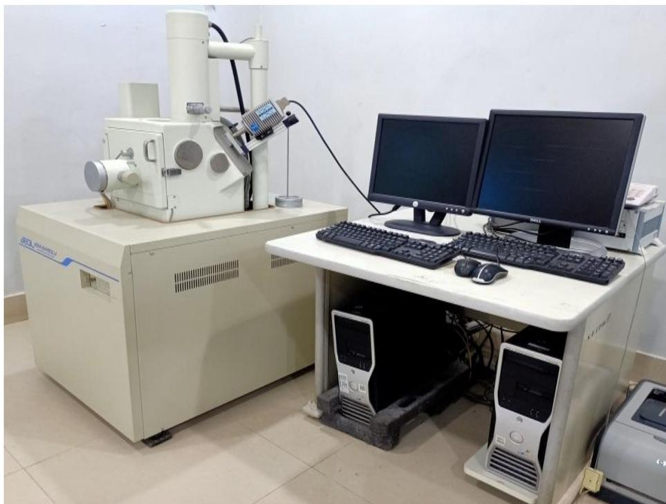
**Figure 2 JEOL JSM-6490 LV for SEM-EDS analysis**
