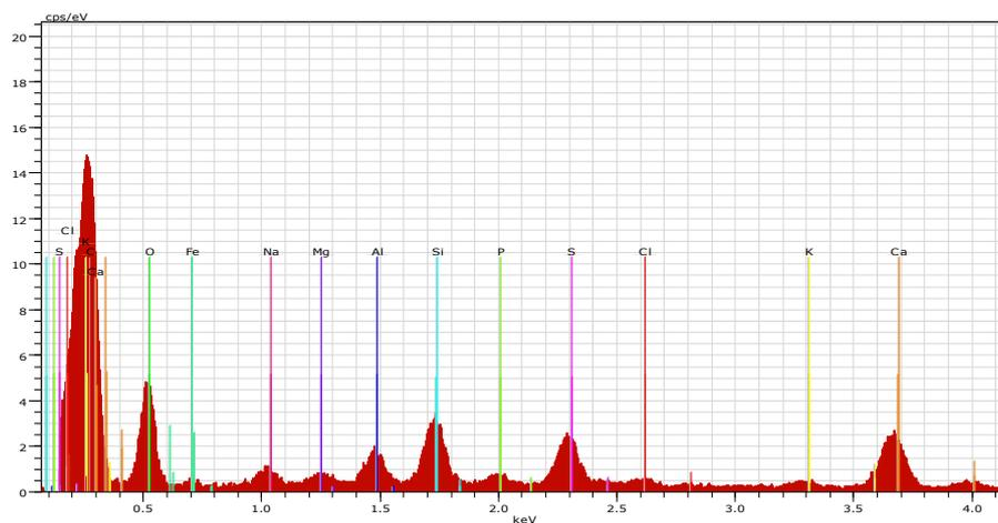
**Figure 7: EDX analysis of inlet valve at CL3000PPM**
