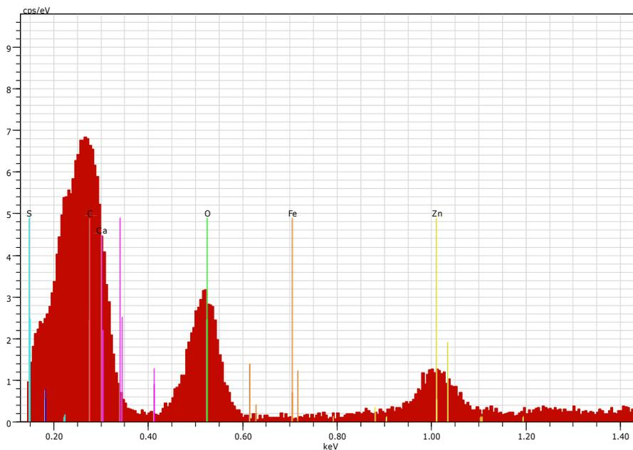
**Figure 4 EDX analysis of inlet valve at D100**
