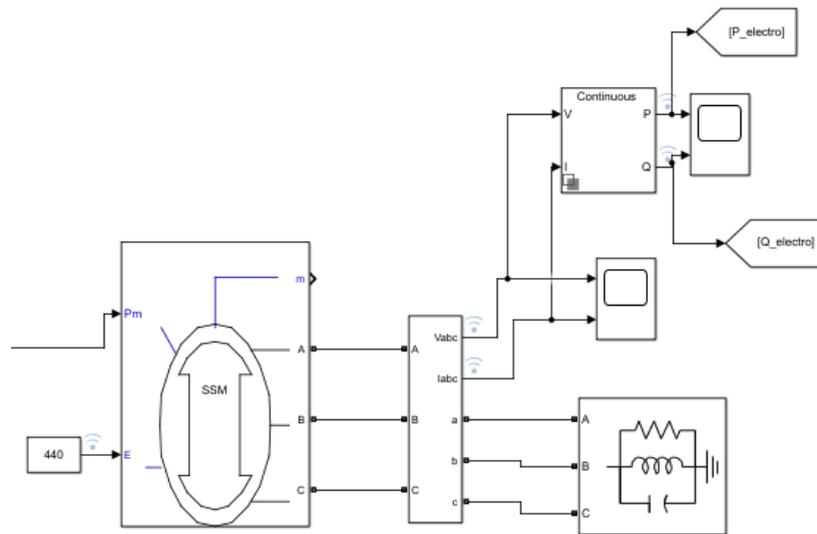
Figure 2.6: 3-Phase Synchronous Generator.
