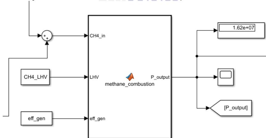
Figure 2.5: Methane Combustion Chamber.
