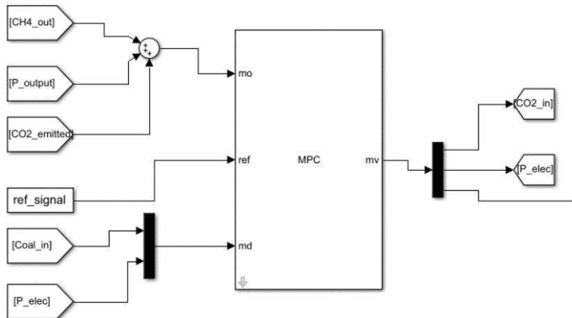
Figure 2.7: MPC Chamber.
