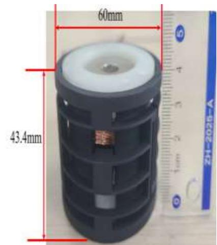
Fig. 33: Fabricated VEMEH [83]
