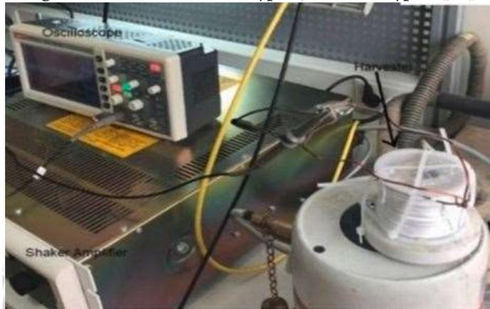
Fig. 24: A non-resonant VEMEH developed [74]
