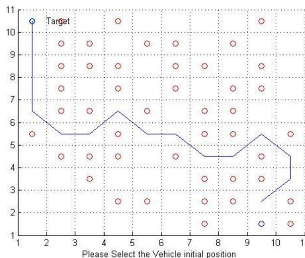
Figure 9: Path Planning for Autonomous Vehicle Navigation in a Grid Environment
