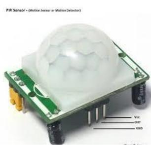
Figure 2: Infrared thermopile array (PIR) sensors
