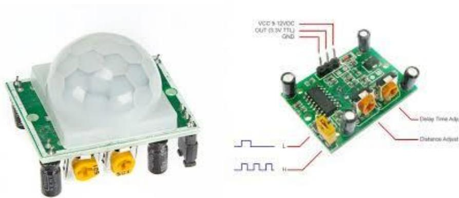
Figure 3: HC-SR501 Passive Infrared (PIR) Motion Sensor Module
