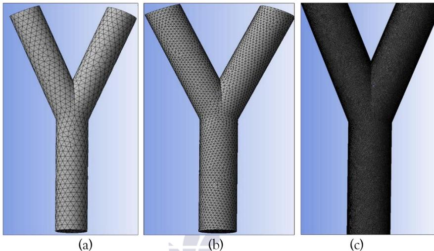
Figure 0.3 Illustrate the mesh size (a) 1 mm (b) 0.5 mm (c) 0.1 mm
