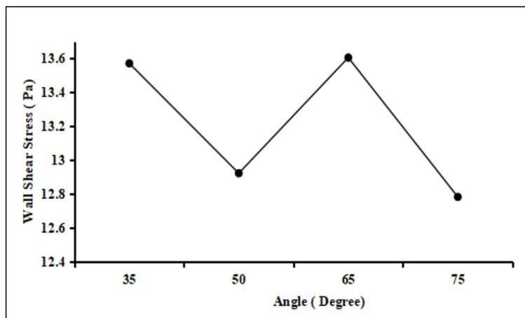
Figure 0.5 Graph between Angles and Wall Shear Stress
