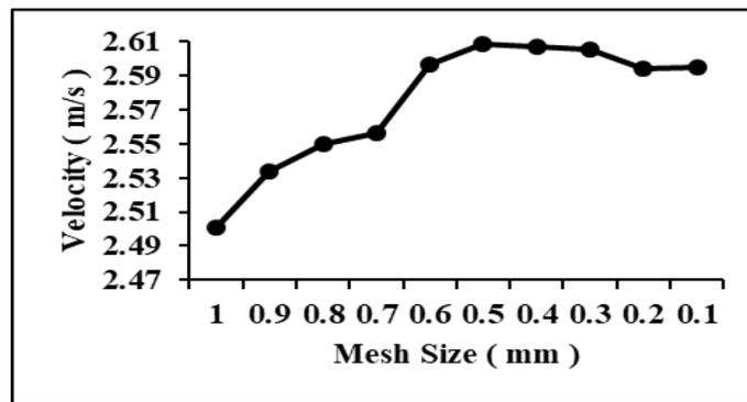
Figure 0.2 Velocity values for Refined Mesh Size
