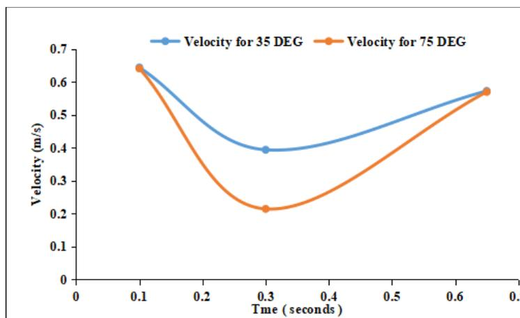
Figure 0.11 Flow distribution between the angles of 35° and 75° with respect to time
