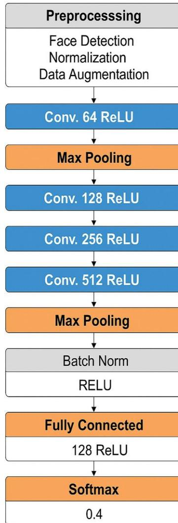
Fig. 3. Model architecture showing various layers, including convolutional layers, pooling layers, fully connected layers, and a softmax layer for classification.
