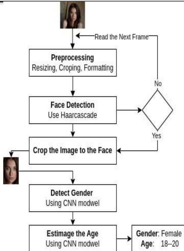
Fig. 2. The algorithm flow diagram. First, face detection followed by gender classification and age estimation.
