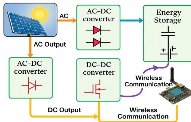
Figure 1. Basic architecture of the Energy Harvesting System (EHS).
