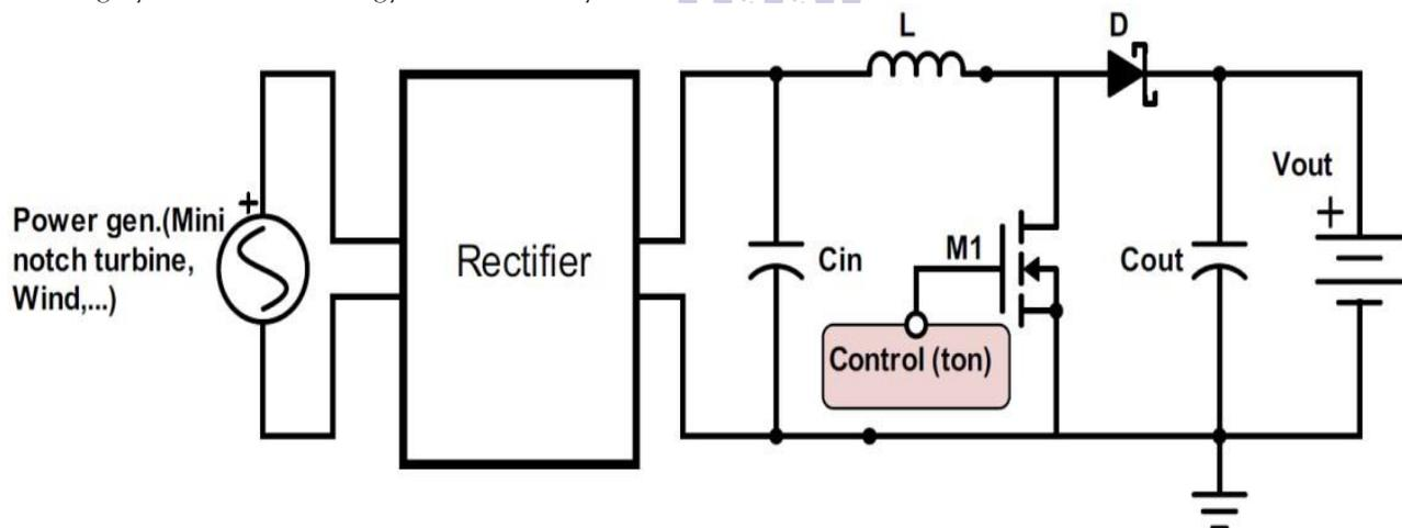
**Figure 13.** MPPT (Maximum Power Point Tracking) utilizing a DC-to-DC boost converter, Illustrating the power optimization process in the system.
