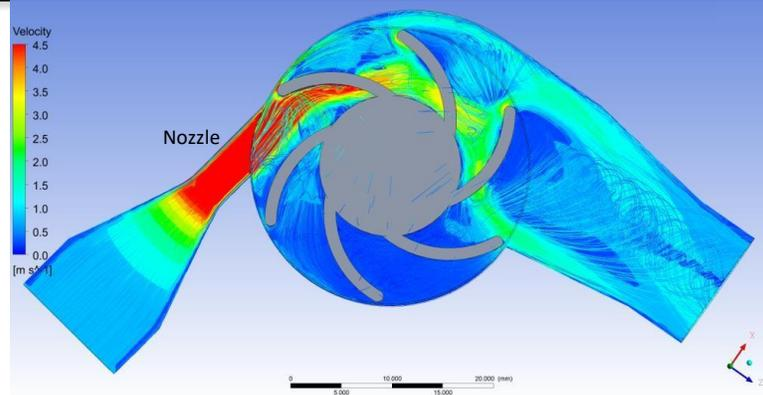
Figure 3: Simulation results of the MiNt nozzle, demonstrating flow characteristics and performance analysis.
