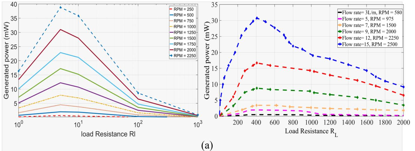
Figure 5: Power curves of the MiNT generator, plotted for various resistance values to show performance variation.
