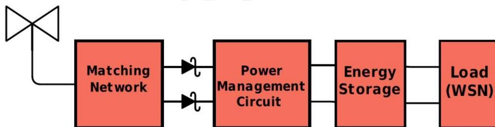
**Figure 8.** An RF energy harvesting system's block diagram illustrates key components and energy flow pathways.
