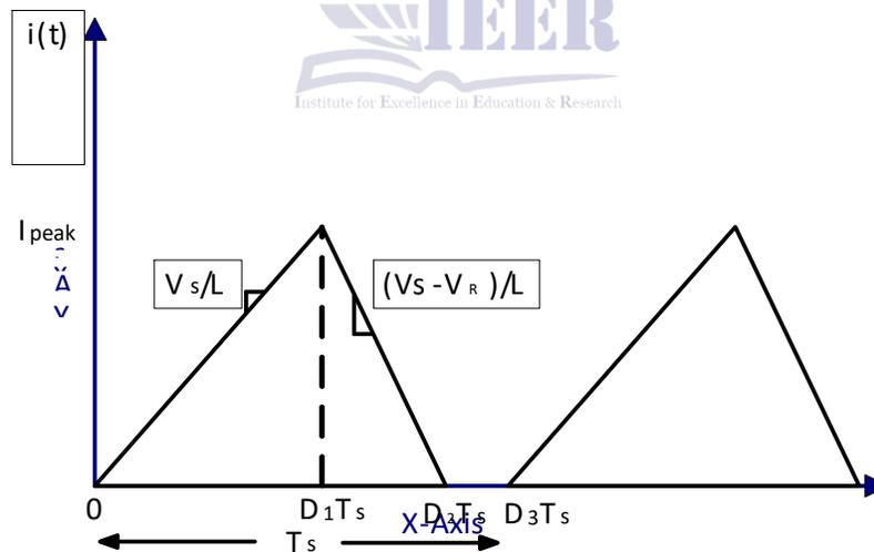
Figure 12: Waveform of the inductor current, depicting its behavior and variations over time.
