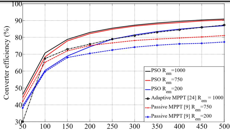
Figure 15. Comparison between PSO and passive MPPT, highlighting performance differences as referenced in [13, 16].
