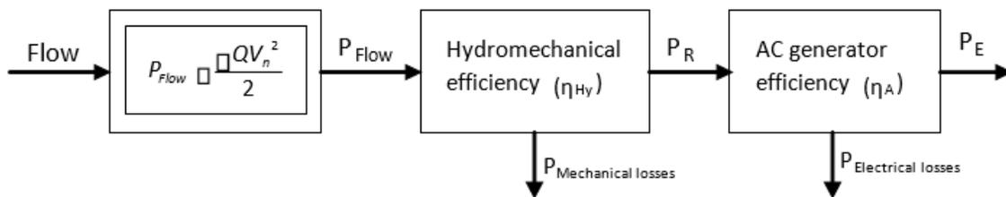
Figure 4: Flow pattern and block diagram of the MiNt turbine, illustrating operational stages and system layout.
