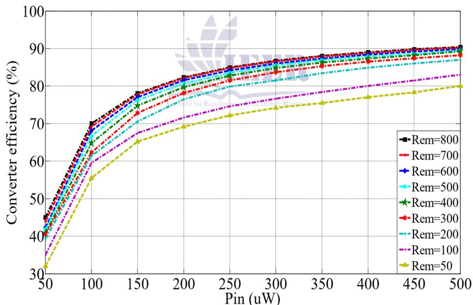
Figure 14. Results of Rem (55-850 Ω) for Pin (55 μW - 550 μW), showing the relationship between input power and the measured resistance.
