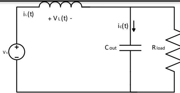
Figure 11. Boost the DC to DC circuit with the MOSFET in the off state, Showing the circuit configuration and energy flow.
