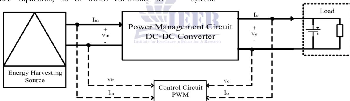
**Figure 9.:** Illustration of impedance matching in an EHS, achieved through a DC to DC converter for efficient power transfer.
