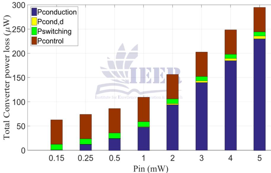
Figure 16. Calculations of power loss for varying input power, illustrating the relationship between input and power loss.
