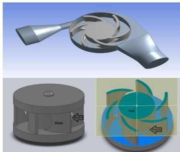
**Figure 2.** The mini-notched turbine's structural configuration highlights its main design features and arrangement.
