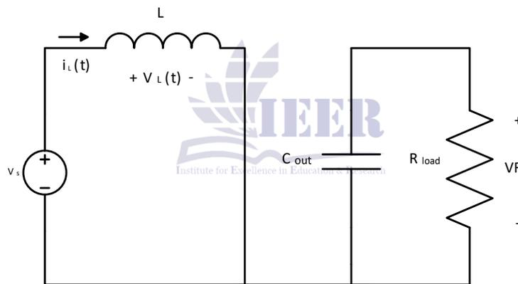
Figure 10. Boost DC to DC circuit when the MOSFET is in the on state.
