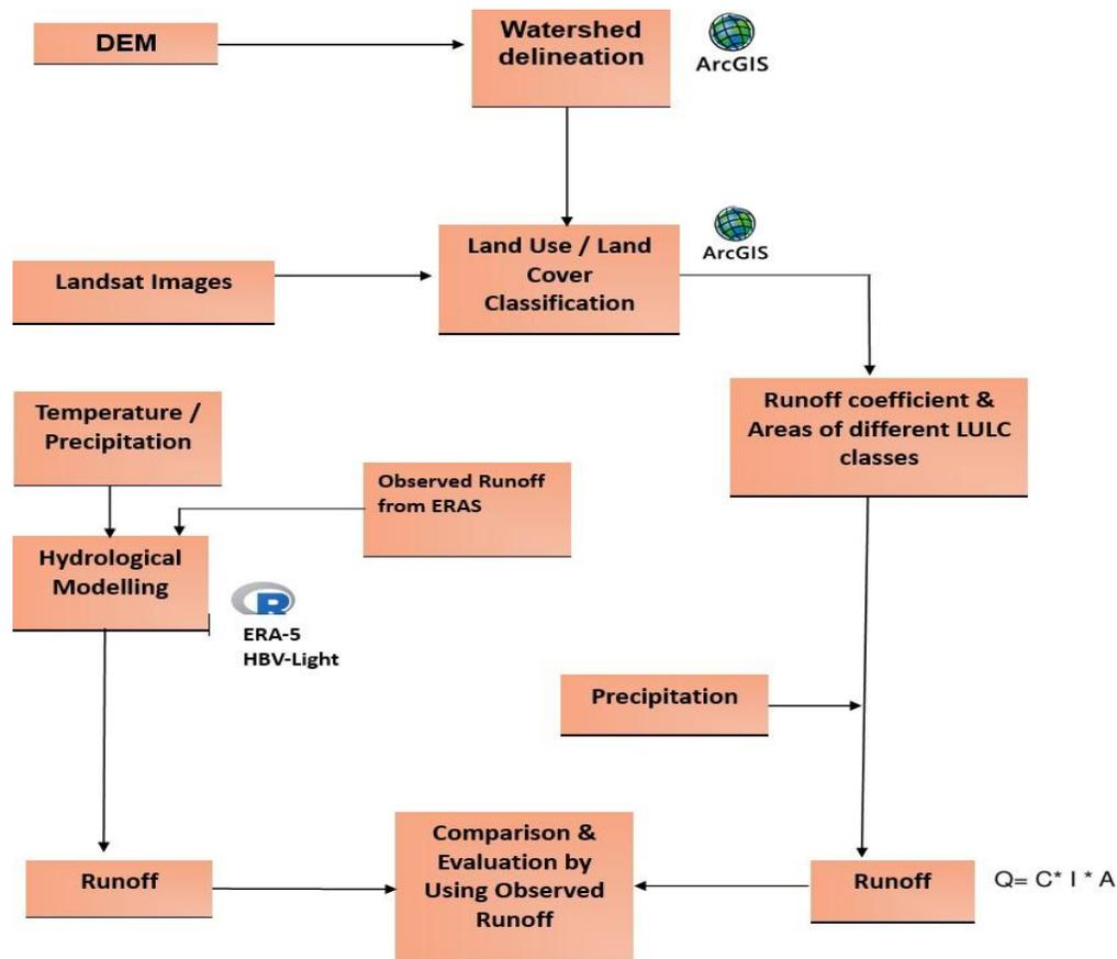
Figure 2: Steps adopted for the calculation of discharge
