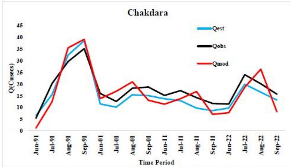
Figure 14: Relationship between  $Q_{est}$ ,  $Q_{obs}$  and  $Q_{mod}$  for Chakdara Sub watershed
