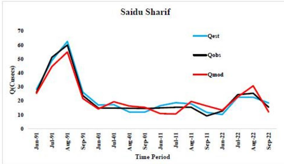
**Figure 15: Relationship between  $Q_{estsr}$ ,  $Q_{obs}$  and  $Q_{mod}$  for Saidu Sharif Sub watershed**
