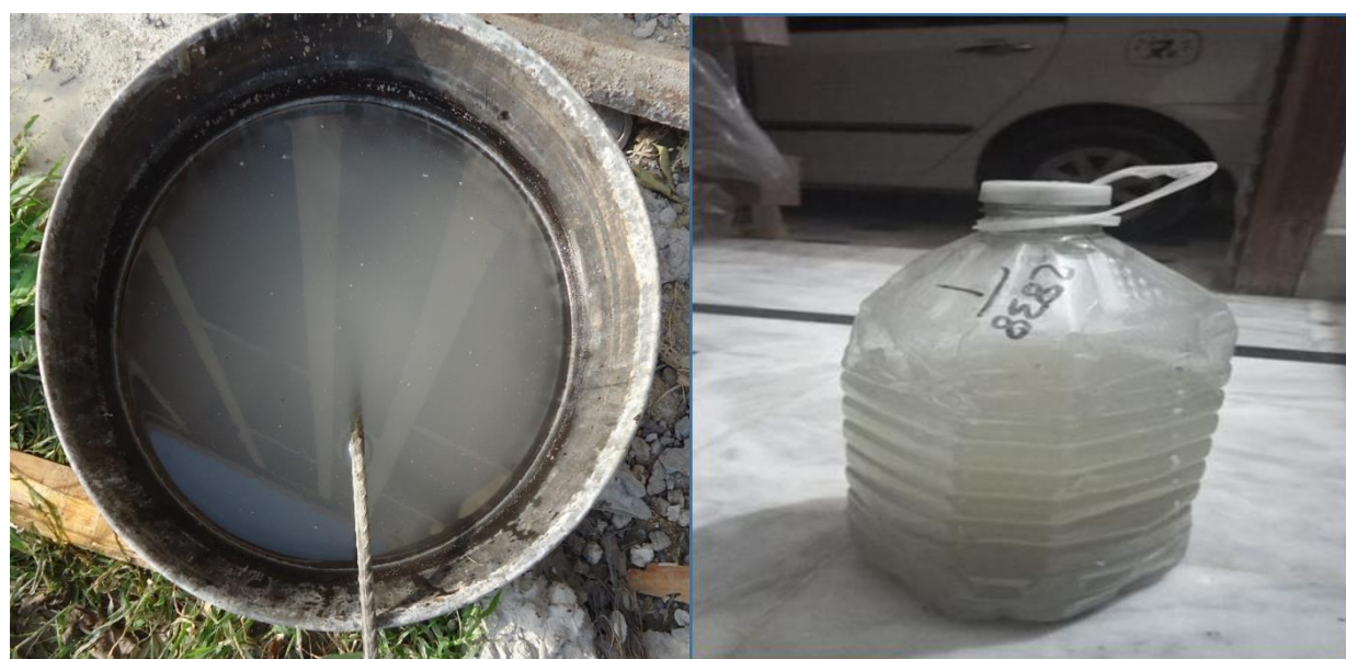
Figure 2: Solution of ( \text{Na}_2\text{SiO}_3 - NaOH) and Sodium Silicate in liquid form
