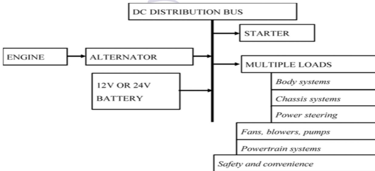
**Figure 6:** Evolution of Power System Architecture in Modern Vehicles [29].
