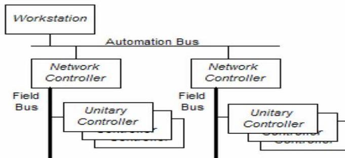
Figure 5: Transition from Point-to-Point Wiring to Fieldbus-Based Architectures [28].
