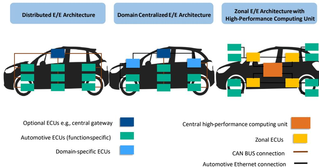
Figure 3: The figure shows how vehicle e/e architecture has changed over time. until 2019, cars mostly used a distributed e/e system. today's vehicles use a domain-centralized setup, and the future will likely use zonal architecture [13].
