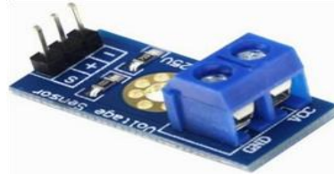
Figure 4 (Voltage sensor ZMP101B)
