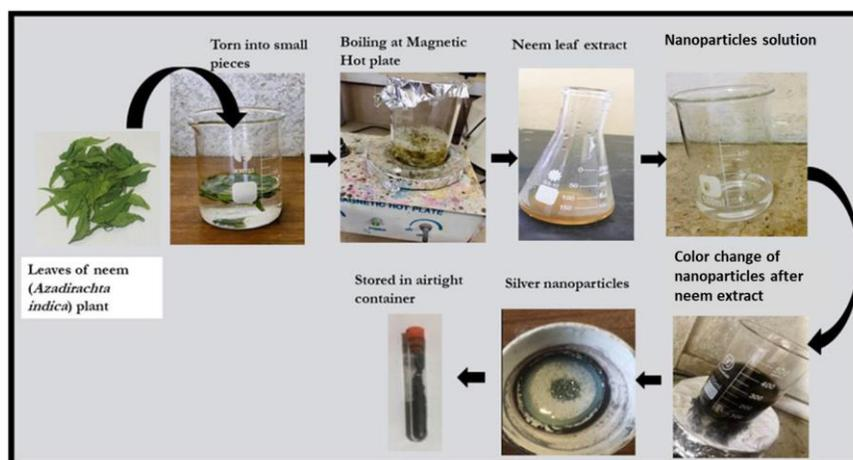
**Figure 1:** Schematic green synthesis of nanoparticles using neem extract
