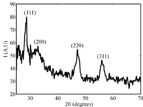
Figure 4: XRD pattern of Nd-doped-ceria nanoparticles.
