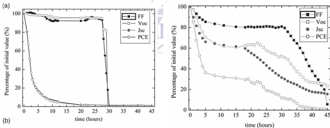
Figure 7: PV characteristics, as a function of exposure time normalized to their initial values for the reference (a) and the Ag NPs-based solar cells (b).
