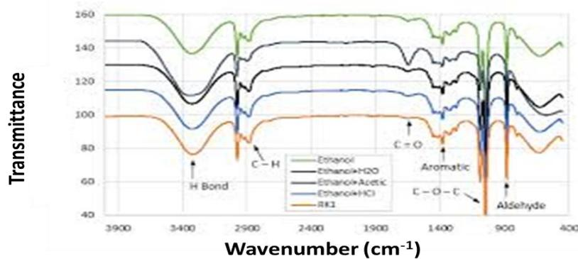
**Figure 2:** FTIR analysis of nanoparticles showing characteristic absorption bands corresponding to various functional groups.
