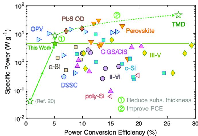
Figure 6: Comparison of photovoltaic technologies: specific power versus power conversion efficiency, emphasizing performance improvement techniques.
