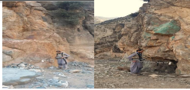
Fig. 4: Field photographs showing acquisition of magnetic data using Geometrics G-858 magnetometer across various alteration zones within the Gawuch Formation.
