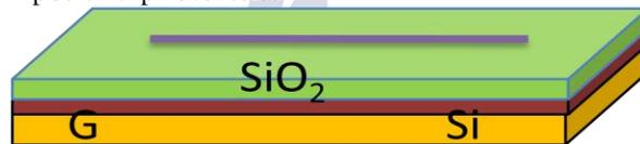
Figure 3: Single GaN-ZnO nanowire aligned between source and drain Ti/Au electrodes on SiO<sub>2</sub>/Si substrate.
